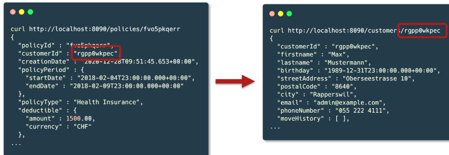
Fig. 14. The customer data can be retrieved by using the customerId in a follow-up request to its Master Data Holder endpoint.
